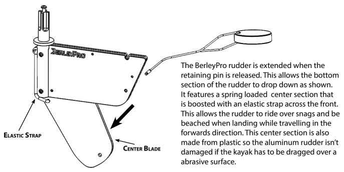
\*Note\* The BerleyPro rudder has been designed with the intention of no metal rubbing on and plastic components. The BerleyPro rudder is susceptible to sand jamming the blade, so take care not to drag the kayak for considerable distances to avoid this. If the blade is jammed you can easily free the blade by hand in the water.
